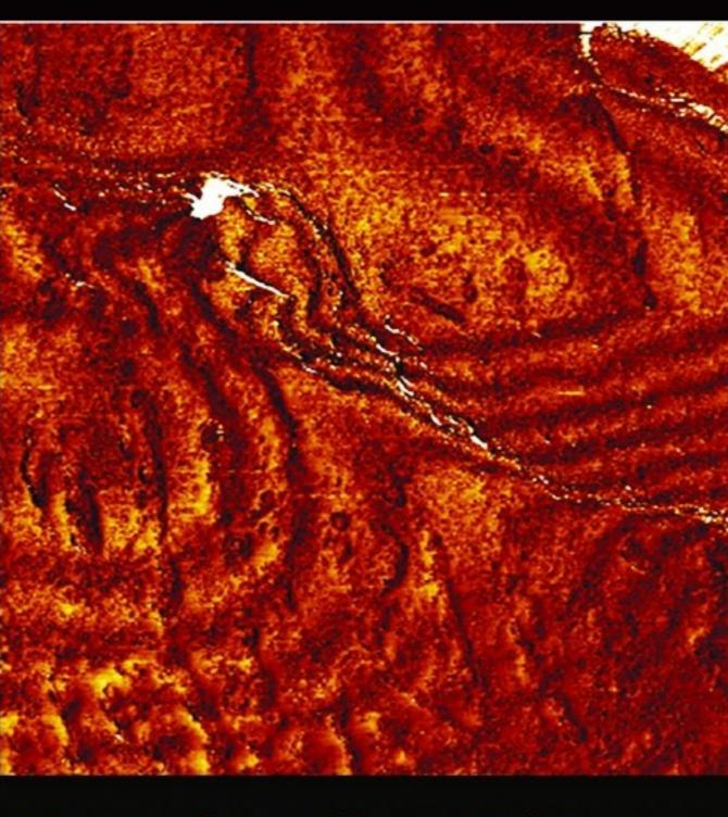
10x10 μm² AFM adhesion image of a cell. Interference artifacts are clearly seen on the PeakForce QNM image.
