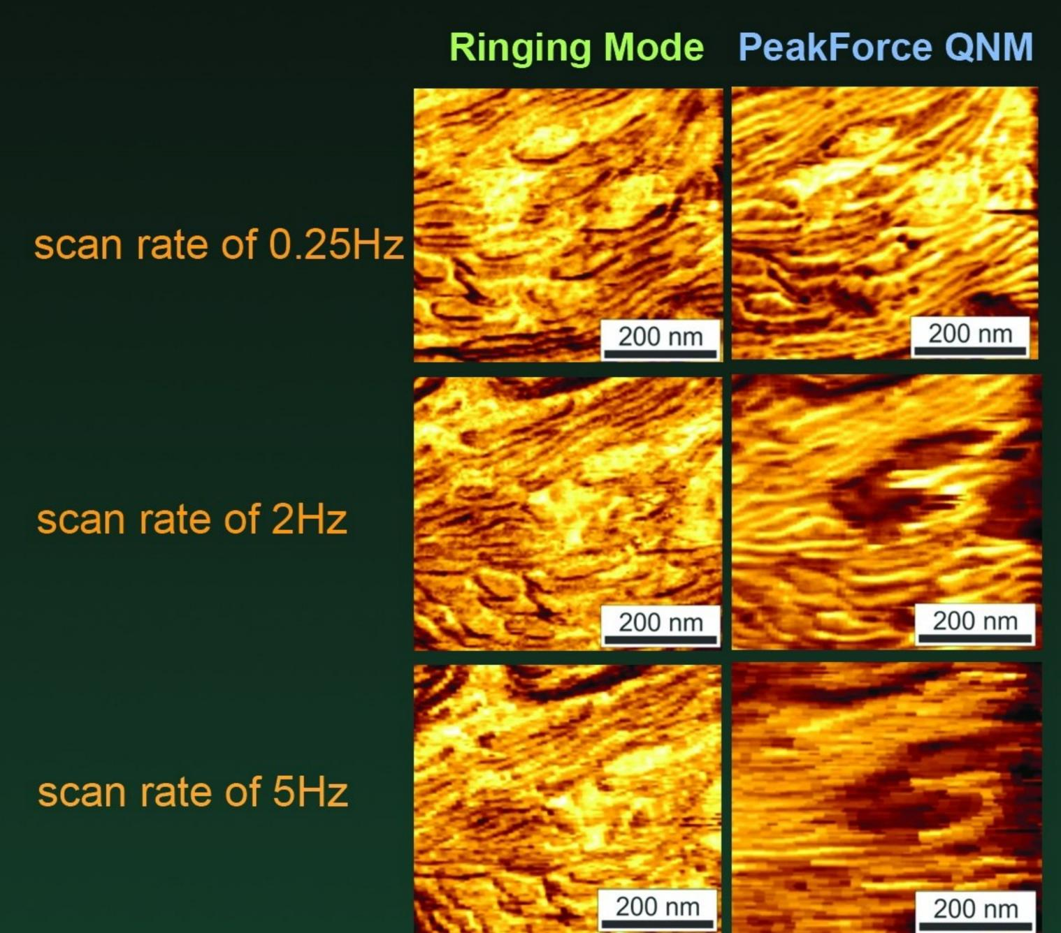
2x2 μm<sup>2</sup> AFM adhesion image of two polymer blend.
